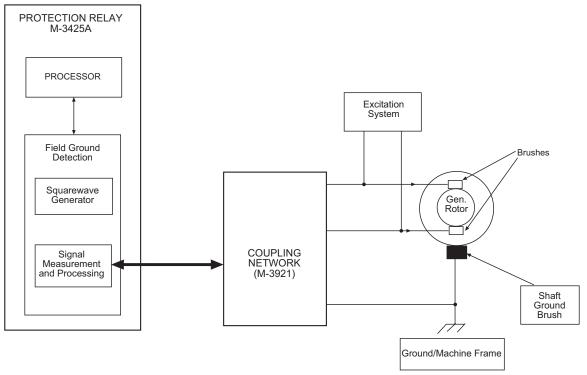
Figure 11 Field Ground Protection Block Diagram
