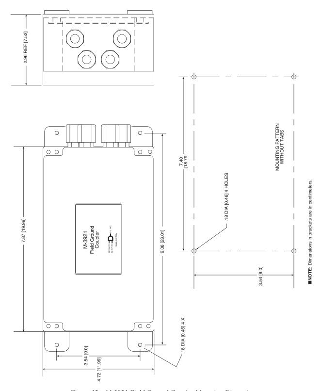
Figure 12 M-3921 Field Ground Coupler Mounting Dimensions
