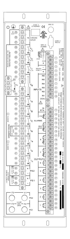
Figure 8 M-3425A Vertical Unit Layout
