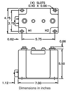
Figure 17 20 Hz Measuring Current Transformer 400-5 A CT
