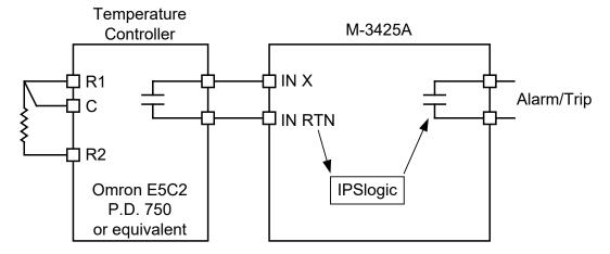
Figure 1 Typical Temperature Controller Monitoring Application
