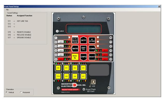
Figure 16 IPScom Smart Button Programming Screen
