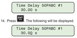
15. Utilizing the arrow pushbuttons enter the desired Time Delay, then press
